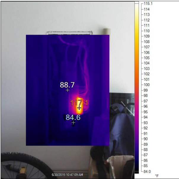
A. Item 3(Picture) Infrared Image of Normal Electrical Panel
